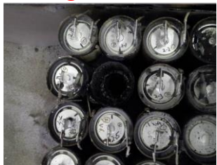
Cell ignition test
